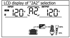
Step 4: Switch on all AC breakers of Line wires in AC input. It's better to connect all of the inverters to the utility at the same time. If not, it will display fault 82 in the following inverters. However, these inverters will automatically restart. If detecting AC connection, they will work normally.
