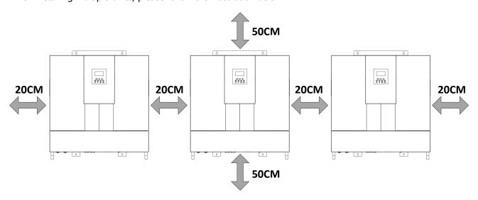
**NOTE:** For proper air circulation to dissipate heat, allow a clearance of approx. 20 cm to the side and approx. 50 cm above and below the unit. Be sure to install each unit in the same height.
