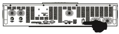
Once the unit has been properly installed and the batteries are connected well, simply press On/Off switch (located on the bottom of the inverter) to turn on the unit.
