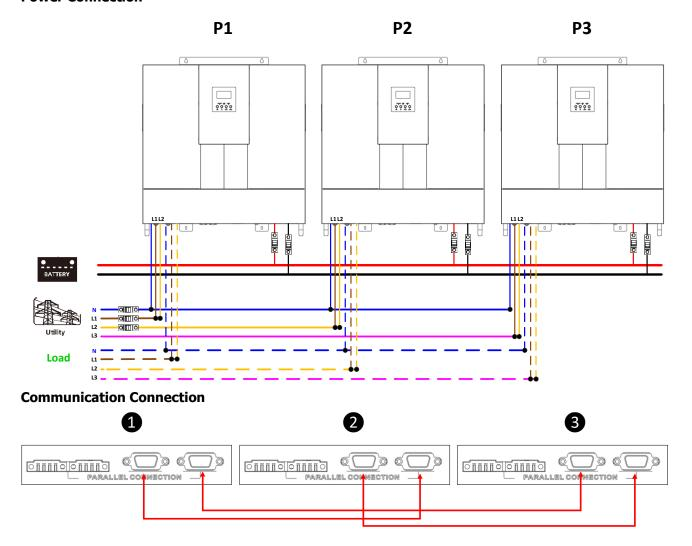
**WARNING:** Do NOT connect the current sharing cables between the inverters in different phases. Otherwise, it may damage the inverters.
