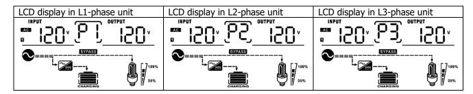
Step 5: If there is no more fault alarm, the system to support 3-phase equipment is completely installed. Step 6: Please switch on all breakers of Line wires in load side. This system will start to provide power to the load.
