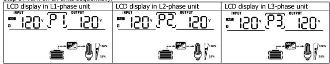
Step 4: Switch on all AC breakers of Line wires in AC input. If AC connection is detected and three phases are matched with unit setting, they will work normally. Otherwise, the AC icon will flash and they will not work in line mode. Under this circumstance, you can switch wires of AC inputs from L2 phase and L3 phase. Or you may exchange the LCD program 28 of P2 and P3 to solve this problem.
